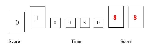
**Error 2:** After finishing the game the puck should be blocked inside the table (doors) If there is no puck in the table (doors) after finishing the game then two middle positions of time display are blinking "**00**".
